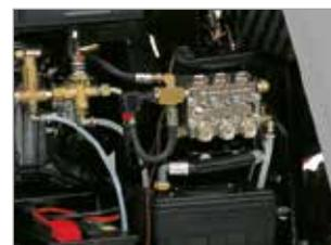
POMPE A PISTONS AVEC TROIS PISTONS EN CÉRAMIQUE ET CULASSE EN LAITON FORGÉE NICKELÉE
